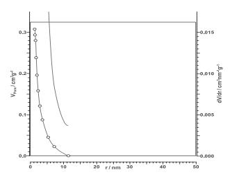
Fig. 3. Pore radius size (nm) vs. pore volume ( $cm^3g^{-1}$ ) in the rice husk silica prepared at 800°C.
