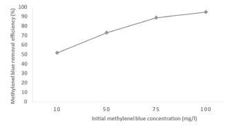
Fig. 7. Effect of the initial methylene blue concentration on the removal efficiency of methylene blue by the rice husk silica.
