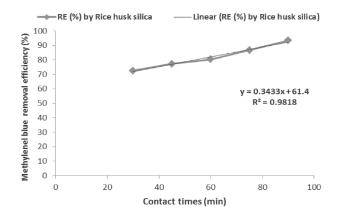
Fig. 9. The correlation between increasing contact times and methylene blue removal efficiency at pH 8, adsorbent dosage of  $1.0 \text{ gl}^{-1}$ , and  $50 \text{ mg}^{-1}$  of the initial concentration of methylene blue by the rice husk silica.
