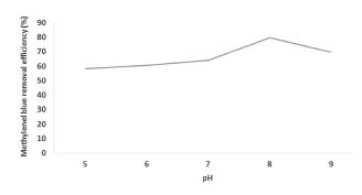
Fig. 6. Effect of the initial solution's pH on the removal efficiency of methylene blue by rice husk silica.
