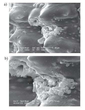
Fig. 4. Scanning electron microscopy (SEM) micrograph of the rice husk silica with magnification of a) 1000 and b) 2000 times.
