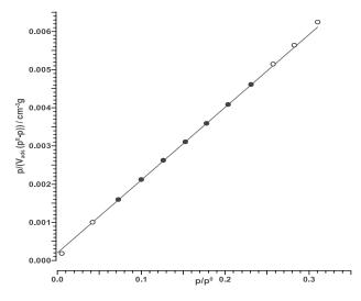
Fig. 2. Surface area (B.E.T.) 2 parameters line  $(p/p^{\circ} Vs. p/(Vads(p^{\circ}-p))/ cm^{-3}g$  in the rice husk silica.
